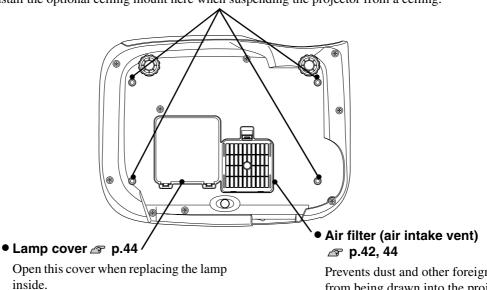
Prevents dust and other foreign particles from being drawn into the projector. It should be cleaned periodically.
